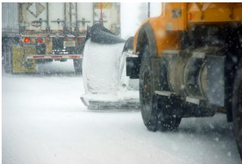
If you are operating in areas with chain laws make sure the chains are in good condition and ready to be installed if needed. Mirrors and all glass in the truck should be clean for maximum visibility.
